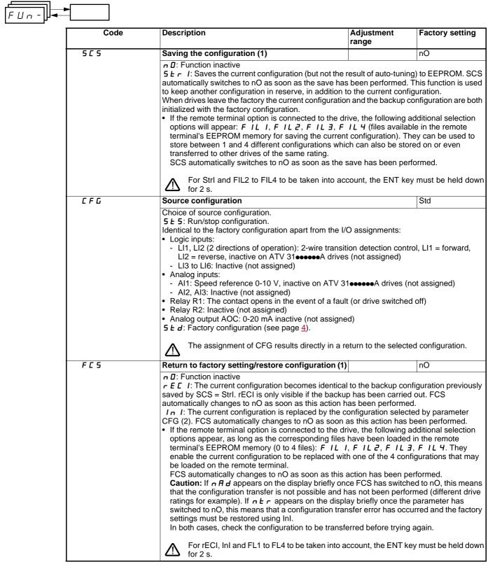
(1) SCS, CFG and FCS can be accessed via several configuration menus but they concern all menus and parameters as a whole. (2) The following parameters are not modified by this function, they retain the same configuration:
