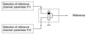
Parameter rFC can be used to select channel Fr1 or Fr2 or to configure a logic input or a control word bit for remote switching of either.
