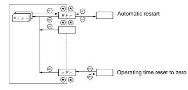
The parameters can only be modified when the drive is stopped and no run command is present. On the optional remote terminal, this menu can be accessed with the switch in the  $\Box^{\cap}$  position.
