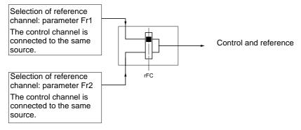
Parameter rFC can be used to select channel Fr1 or Fr2 or to configure a logic input or a control word bit for remote switching of either. See the detailed diagrams on pages <u>35</u> et <u>37</u>.
