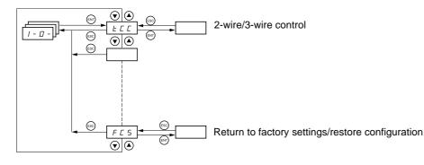
The parameters can only be modified when the drive is stopped and no run command is present. On the optional remote terminal, this menu can be accessed with the switch in the  $\Box^{\cap}$  position.
