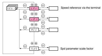
The adjustment parameters can be modified with the drive running or stopped.
