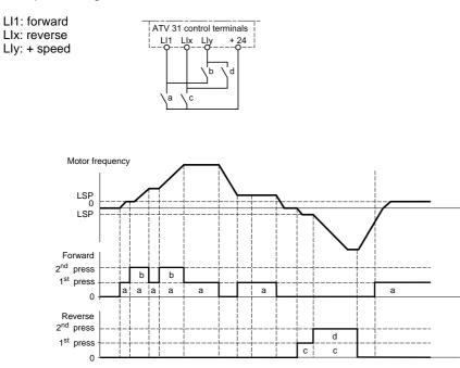
This type of +/- speed is incompatible with 3-wire control.
