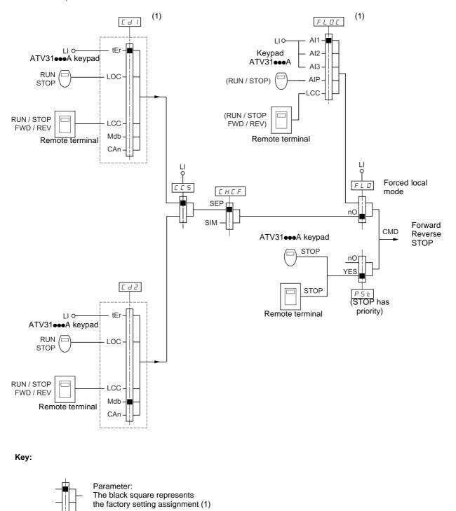
(1) Except for ATV31 ••• A: Cd1 is factory-set to LOC and FLOC is factory-set to AIP.
