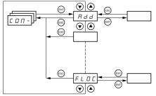
The parameters can only be modified when the drive is stopped and no run command is present. Modifications to parameters Add, tbr, tFO, AdCO and bdCO are only taken into account following a restart. On the optional remote terminal, this menu can be accessed with the switch in the  $\Box$  position.
