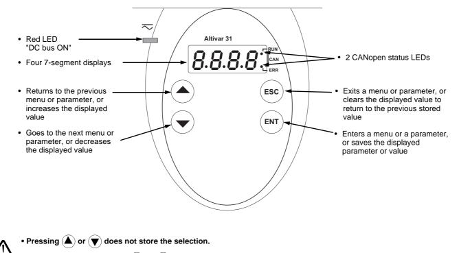
• Press and hold down (>2 s) ( $\blacktriangle$ ) or (igvee) to scroll through the data quickly.
