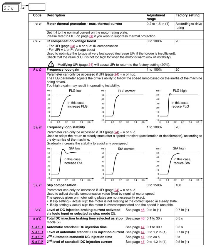
(1) In corresponds to the nominal drive current indicated in the Installation Manual and on the drive rating plate. (2) Caution: These settings are not related to the "automatic standstill DC injection" function.
