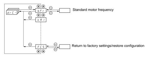
With the exception of tUn, which can power up the motor, parameters can only be modified in stop mode, with no run command present.
