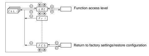
The parameters can only be modified when the drive is stopped and no run command is present. On the optional remote terminal, this menu can be accessed with the switch in the  $\cap$  position.
